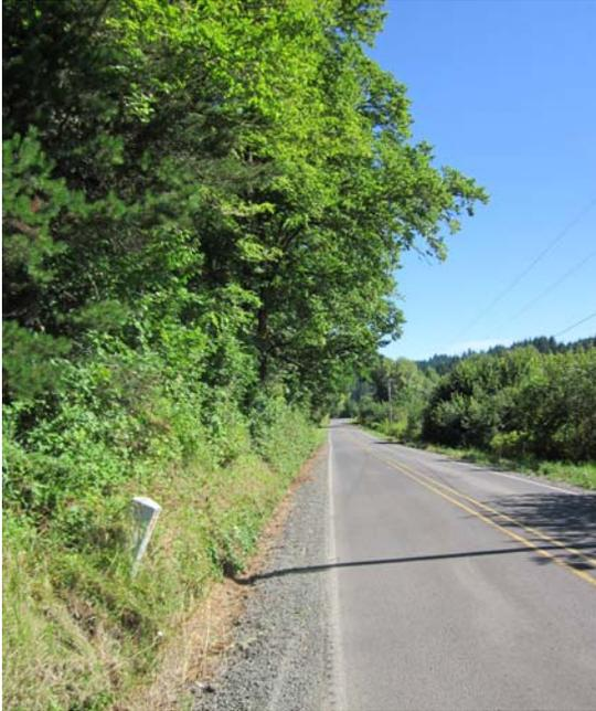
Photo 1: Trees are a consistent distance from the road, outside of an established clear zone.
