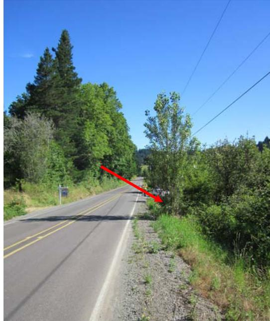
Photo 2: Cottonwood tree is growing in an otherwise clear zone. Removing the tree would re-establish a consistent clear zone.
